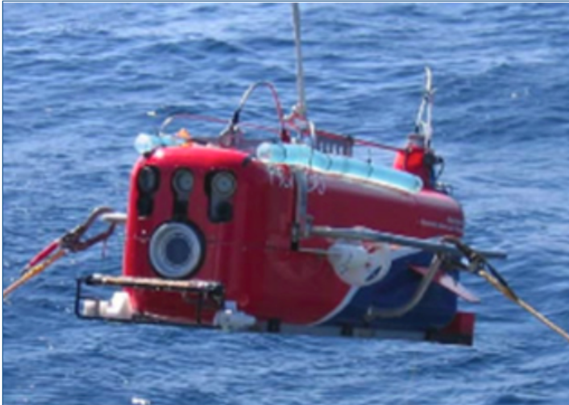
Figure 2. Plankton Investigatory Collaborating Autonomous Survey System Operon (PICASSO). Outfitted with high vision camera, plankton recorder, CTD and sensors.
