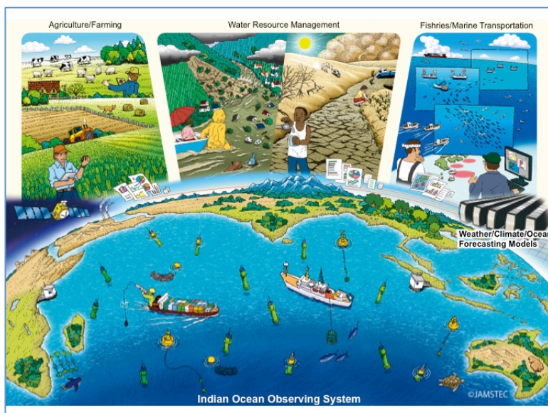
Figure 4: Schematic of ocean observing system in the Indian Ocean and its values for socio-economic applications. Data obtained by the observing system with various instruments are delivered to users directly or indirectly through weather/climate/ocean forecasting
