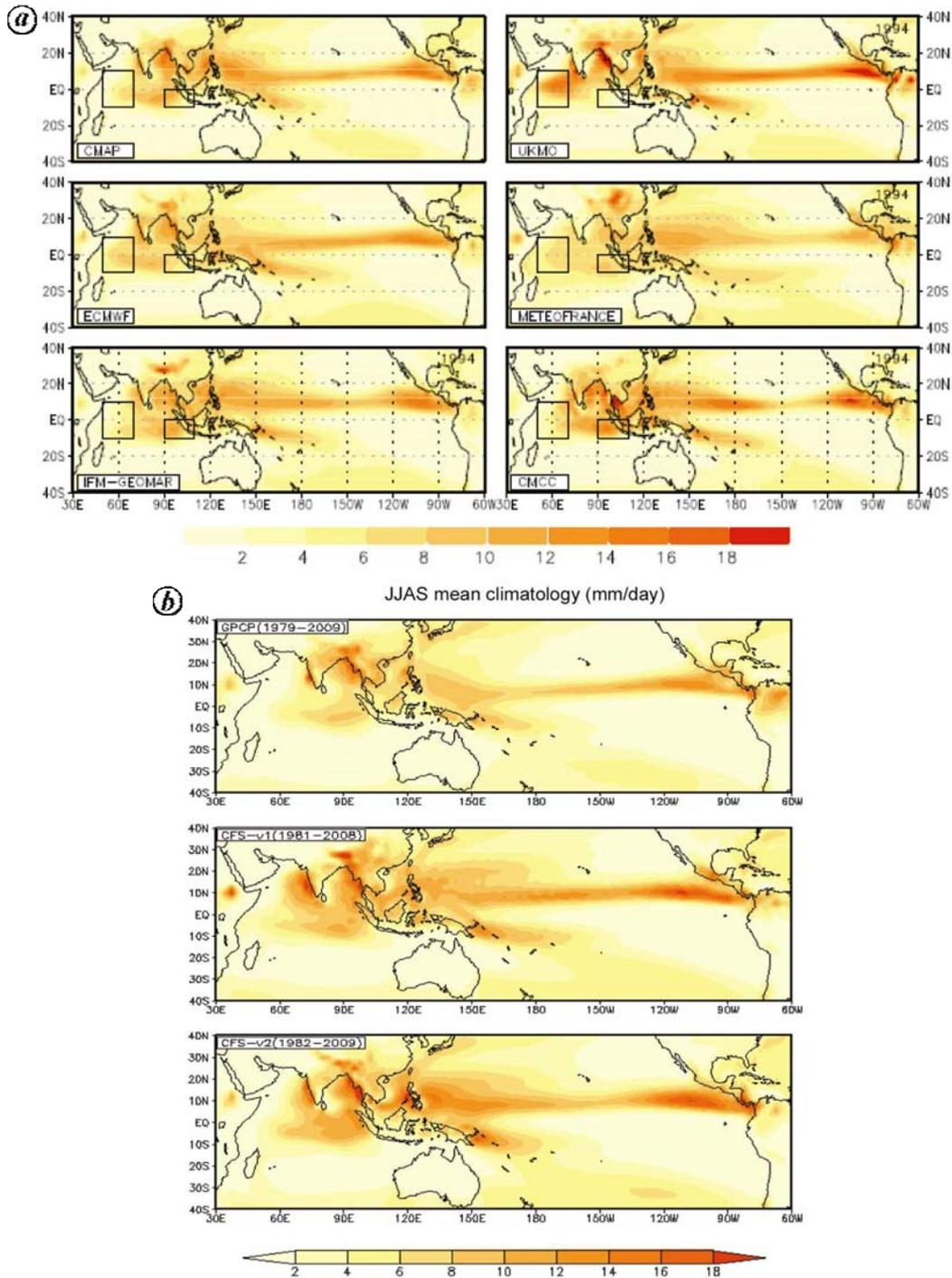
**Figure 5.** *a*, Mean JJAS rainfall patterns from observations (CMAP) and those simulated by five models which participated in the ENSEMBLES project. *b*, Mean June–September rainfall (mm/day) patterns observed (GPCP) and simulated by CFS1 and CFS2.
