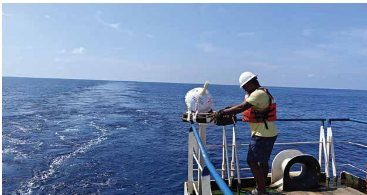
Figure 6.4. INCOIS scientist is deploying an SVP drifter from Sagar Nidhi in the Bay of Bengal
