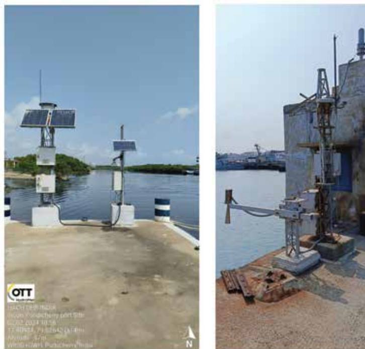
Figure 6.11. The newly installed radar tide gauge stations in Gujarat and Chennai
