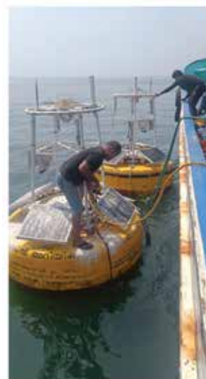
Figure 6.14. Deployment and recovery of coastal observatory at Kochi coast
