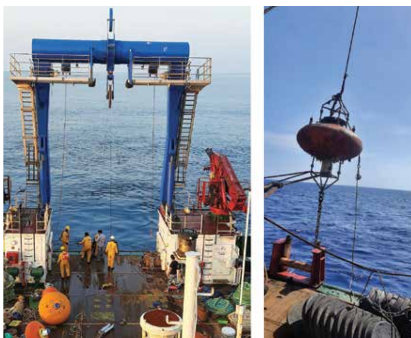
Figure 6.6. Deployment and recovery of equatorial current meter array
