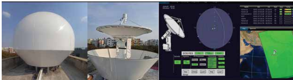
Figure 4.4.9 2.4 m X/L band antenna & Satellite tracking and processing system
