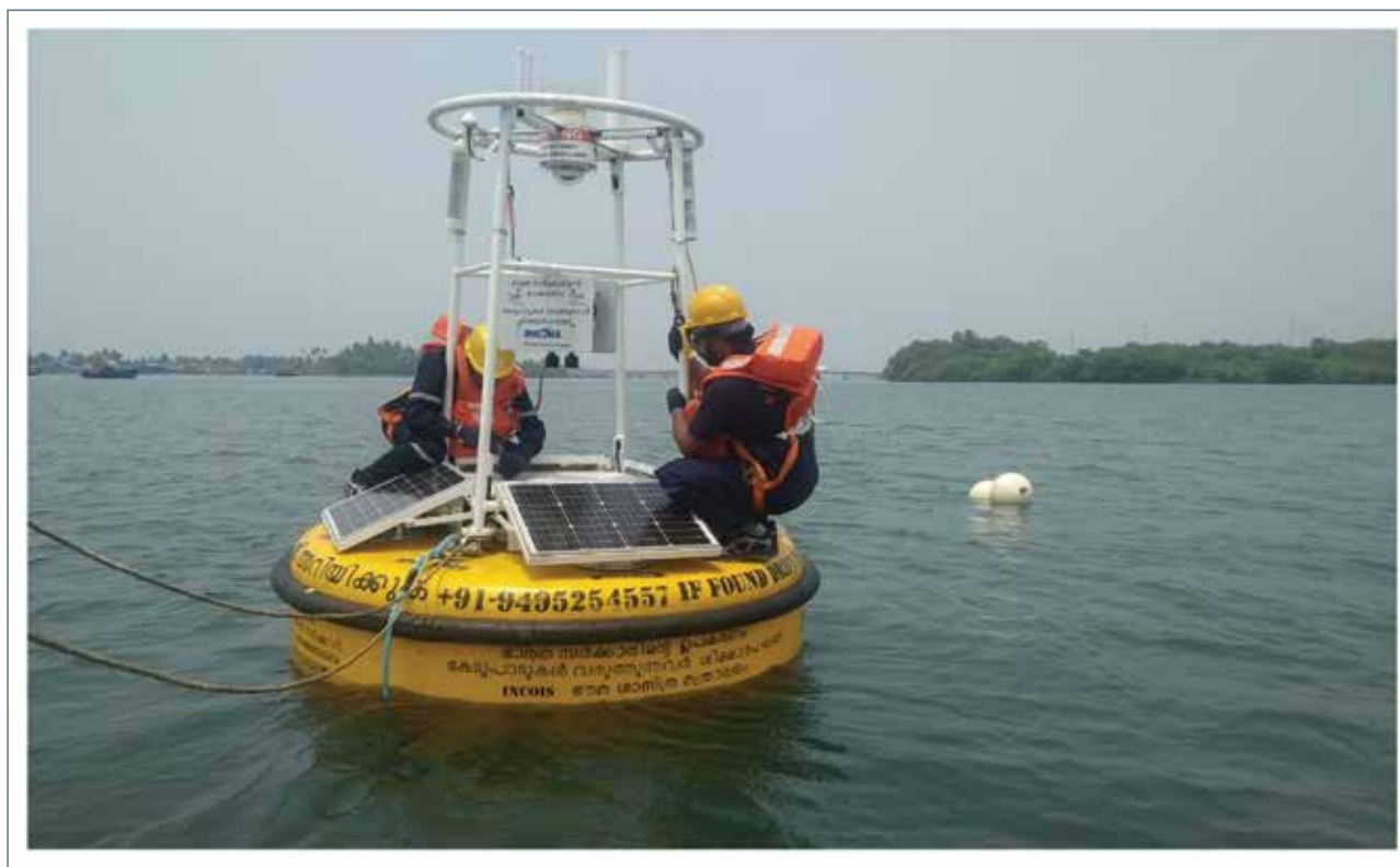
Fig. 6.19 Test deployment of the water quality monitoring buoy in the estuarine region off Kochi on 03 March 2022.
