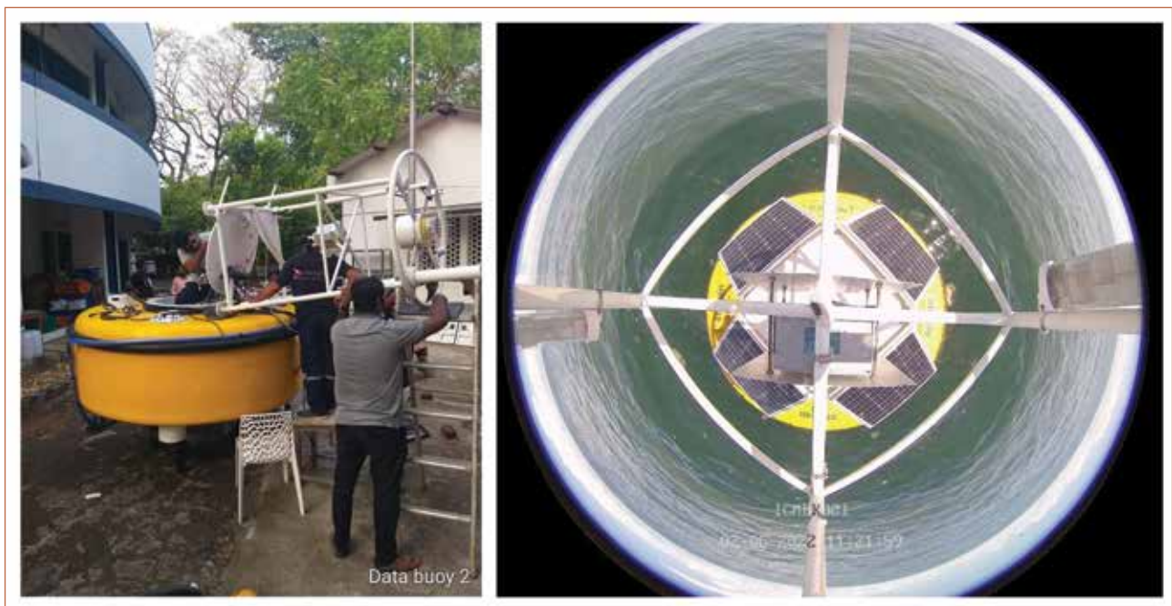
Fig. 4.33 Coastal Buoy Installation, testing of Communication channels (INSAT & GPRS)
