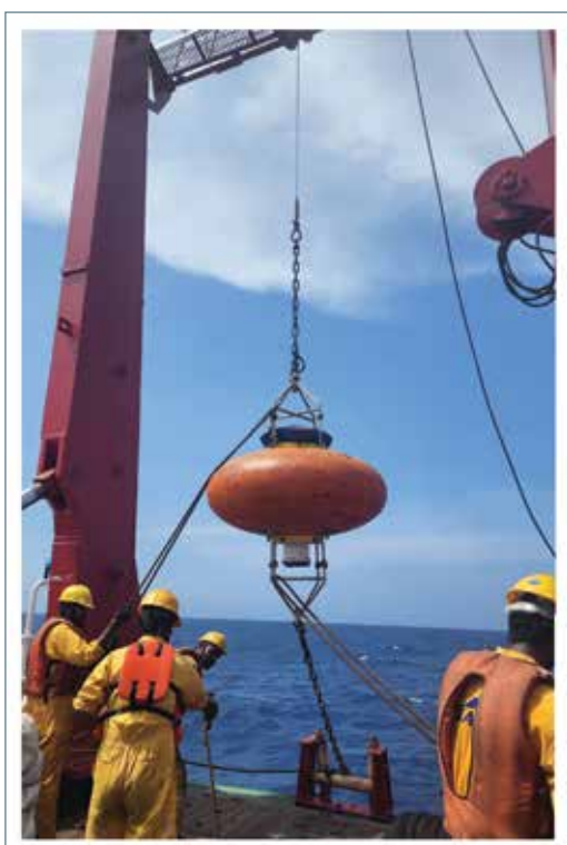
Fig. 6.15 Re-deployment of an ADCP mooring (after service) on the continental slope along the west coast of India during RV Sindhu Sankalp (SSK-140) cruise.
