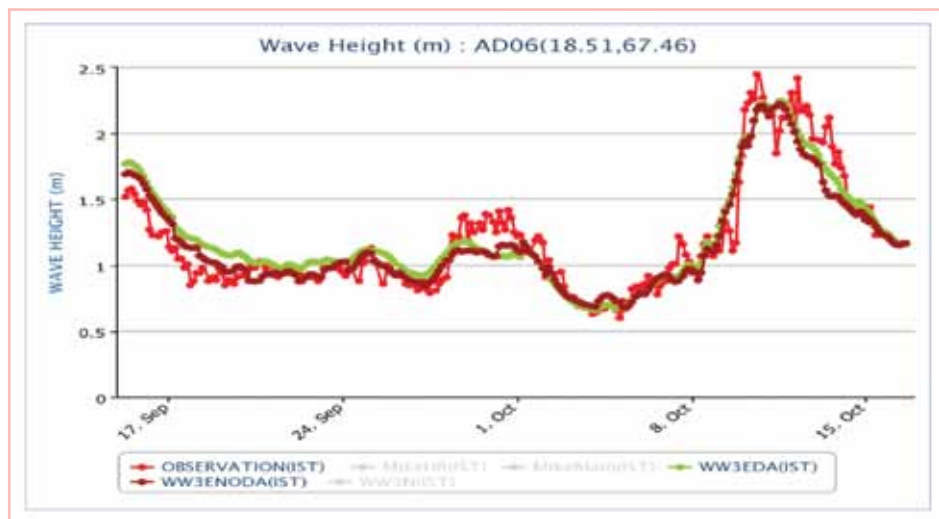
Predicted and Observed wave heights (m) during Cyclone Luban (7-14, October 2018).
