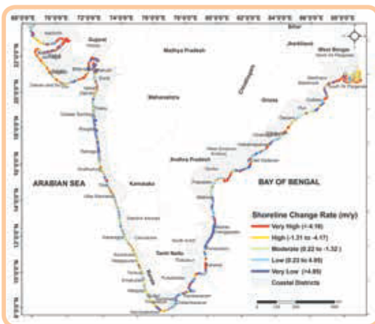
Figure 1: Spatial distribution of shoreline change rate and SOI tide gauge station (asterisk mark) along the Indian mainland coast (negative sign indicates the erosion, and positive sign accretion)
