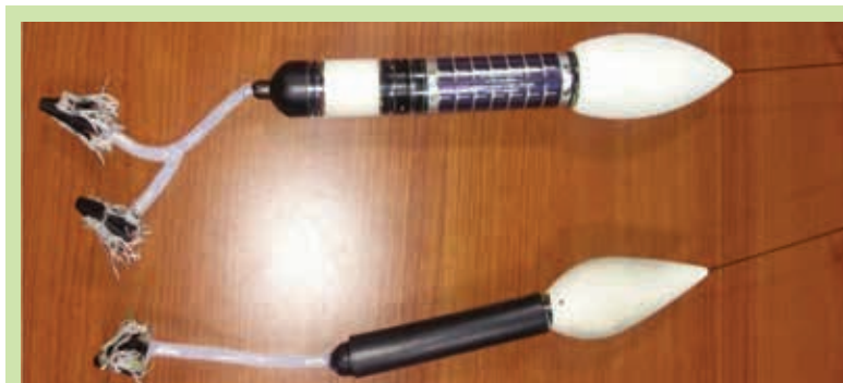
Newly procured PSAT tags with magnetometer, and (in bigger tag) accelerometer
