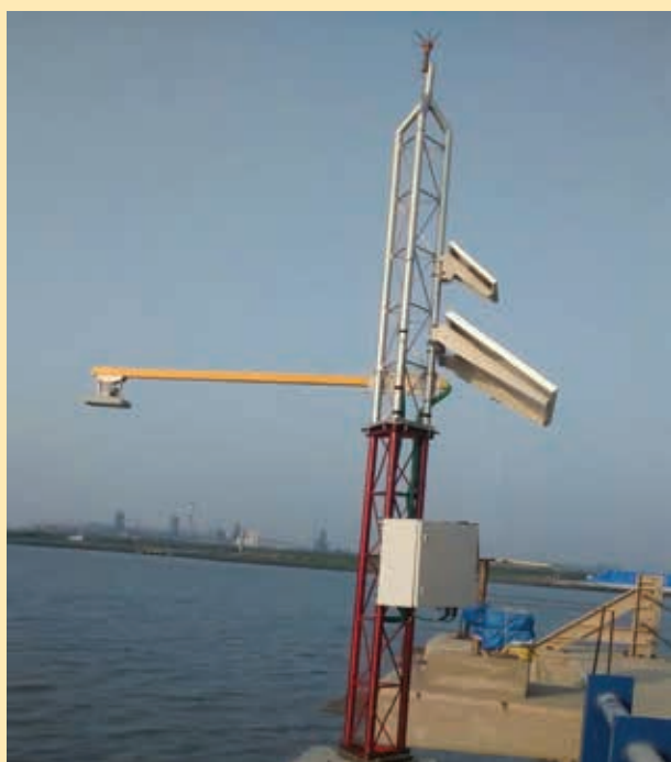
New radar tide gauge stations at Adani Hazira (Left) and Marmagao (Right)
