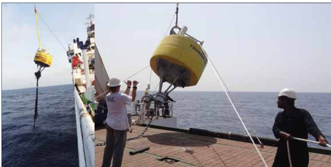
Retrieval and redeployment of the SAIC Tsunami Buoy (STB02) in the Arabian Sea
