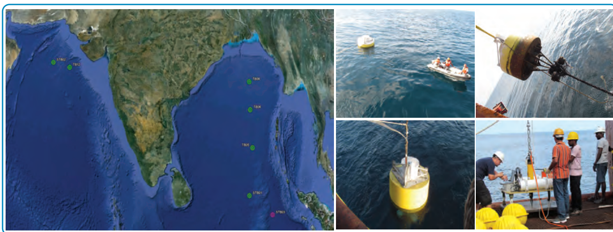
Figure 8.4: (left) Tsunamis buoys network in the north Indian Ocean. Retrieval (middle) and redeployment (right) of the SAIC Tsunami Buoy in the Arabian Sea.
