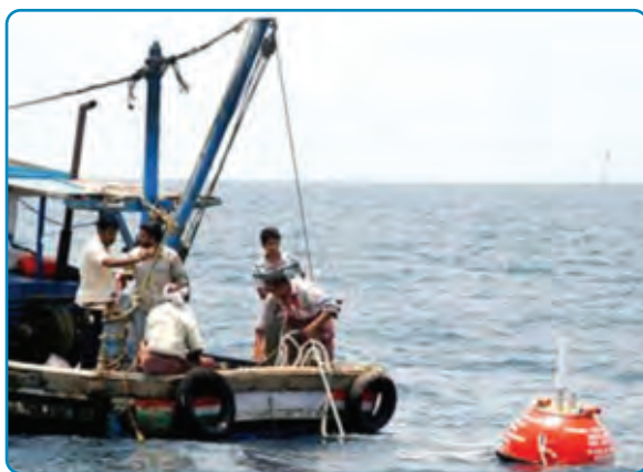
Figure 8.9: Deployment of wave-rider buoy off the coast of Gopalpur, Odisha.
