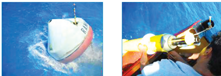
Deployments of (left) second phase of BoB mooring and (right) Iridium-ARGO float
