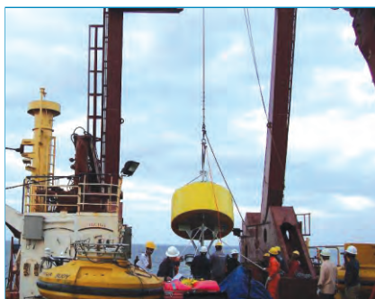
Deployment of Surface buoy and bottom pressure recorder
