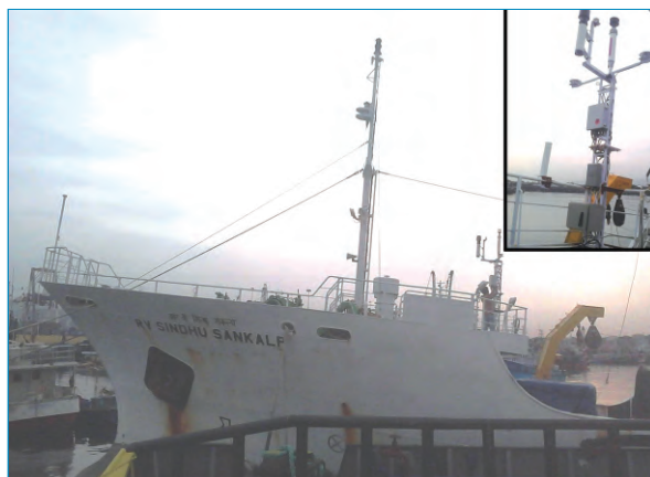
AWS onboard RV Sindhu Sankalp (Inset: close-up view of the AWS)
