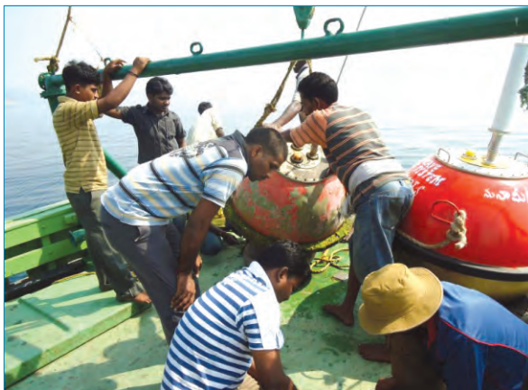
Deployment of wave rider buoy off Visakhapatnam
