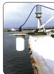
AWS on board Sagar Kanya (left), Deployment of Sediment trap from Sagar Kanya (middle), Wave height meter on board Sagar Nidhi (right).
