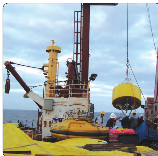
Deployment of the SAIC tsunami buoy in the Arabian Sea Bottom Pressure Recorder: Left and Surface Buoy: Right.
