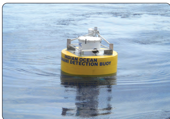
SAIC tsunami buoy deployed in the Bay of Bengal (left) and a Wave rider buoy being deployed in the coastal waters (right).
