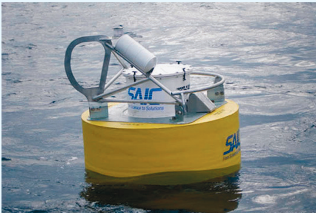
SAIC buoy, STB-01. The data from this buoy deployed west of Andaman Islands at 6.25 °N, 88.65 °E, is being received at INCOIS in real-time through iridium communication link
