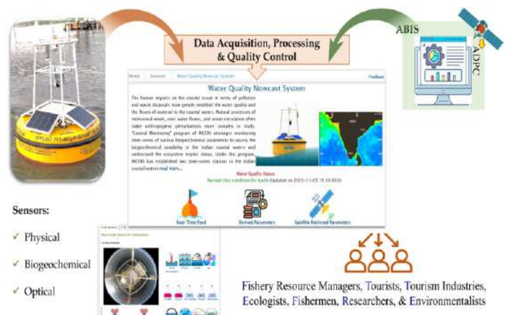
Schematic showing a detailed overview of INCOIS's Water Quality Nowcasting System
