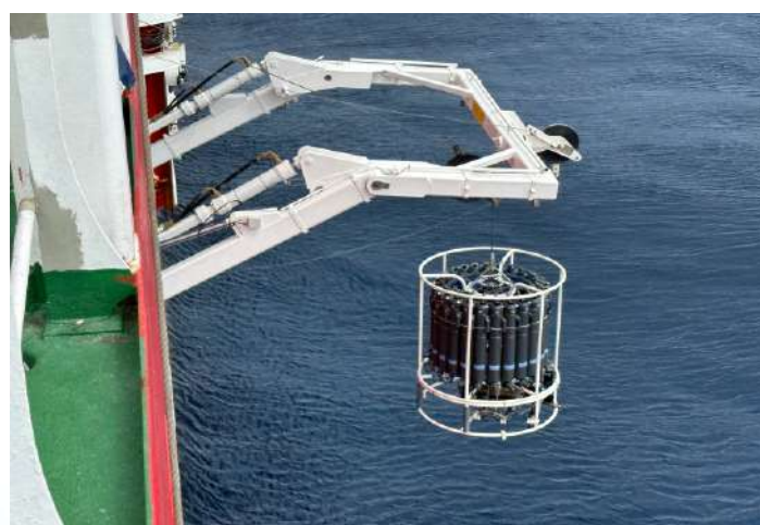
S.A. Agulhas II deploying a CTD along the route from Reunion to Aldabra
