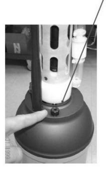
rotate counter -clockwise to unscrew plug.
