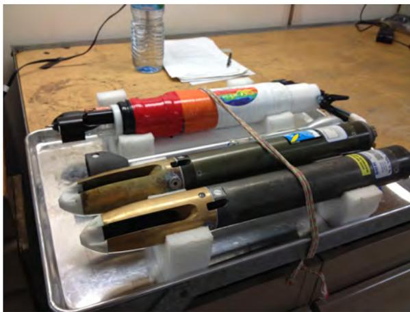
Figure 2: UCTD probes (closest to camera) and JCTD probe (furthest from camera). The JCTD was rigged after we damaged a number of SBE UCTD probes. JCTD, in addition to measuring conductivity, temperature, and pressure, was also equipped with a  $\chi$ -pod to measure temperature microstructure.
