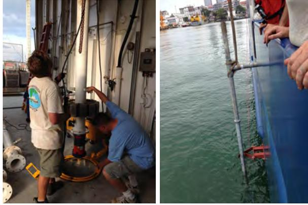
Figure 4: Left: "pipe string" system for installing an additional 300 kHz ADCP in a well in the staging bay. Right: pole system for mounting the Sentinel V ADCP over aft port side of the deck. The instrument was approximately 1 meter below the surface.
